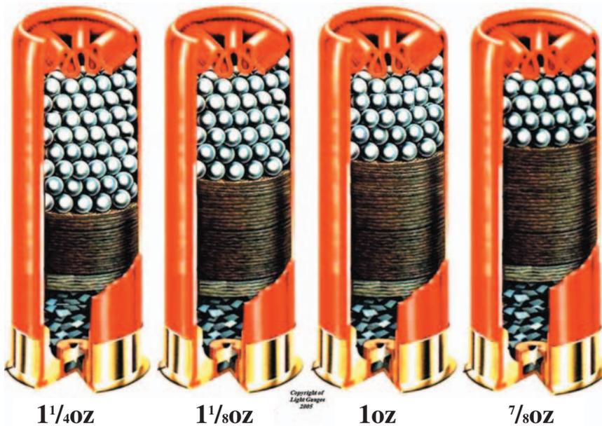
**PROGRESSIVELY INCREASING DOWN THRUST FORCES SHOWING THE INCREASED DISTORTION OF THE SHOT WITH A LONGER COLUMN**
